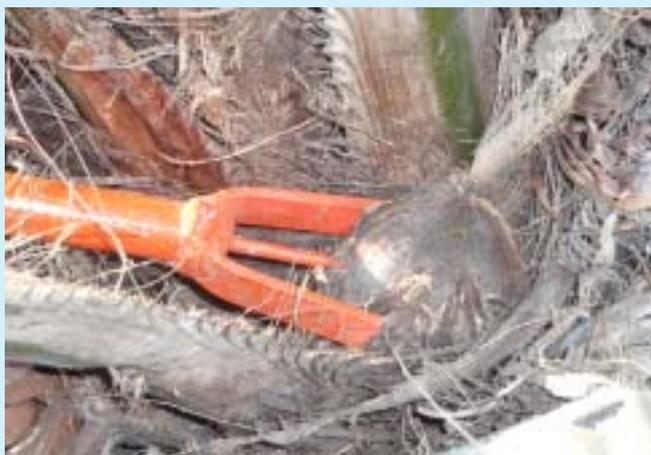
the inflorescence and with a small push, inflorescence gets broken and is hooked like a fish. This tool can generally be operated without drudgery at an angle of 68° with respect to the ground level from a distance of 1.3 m. The average time taken to ablate one inflorescence would be 2.0 seconds. On an average, a worker can ablate 125 inflorescences per hour. Cost of this tool would be less than Rs. 250/-.
