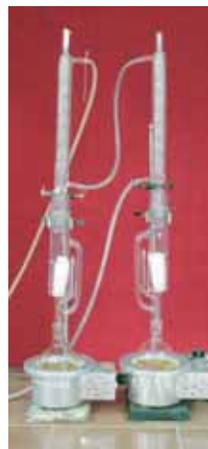
Extraction of oil in Soxhlet apparatus
